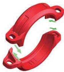
**T&G design:** The T&G (tongue & groove) mechanism provides a mechanical and frictional interlock resulting in a rigid joint which reduces undesired angular movement. WINGROU precision casting techniques allow the coupling segments to meet metal-to-metal when installed on properly grooved pipe.
