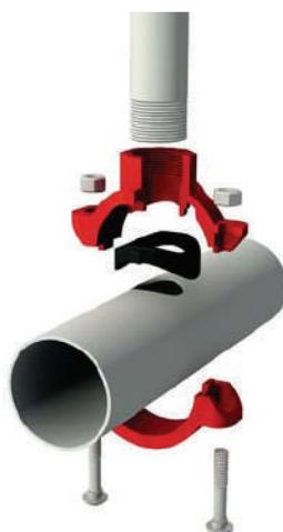
Care should be taken to maintain the area of around 16mm outside the hole (quota s), along with the section of the tube of length L, free of burr, grease, dirt etc., with the aim of achieving total sealing. The coupling should sit perfectly
