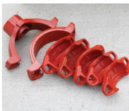
Ductile Iron: Standard coupling housing and fittings are made of ductile iron confirming to ASTM A536 Gr. 65-45-12. The properties of Grade 65-45-12 ductile iron are as follows; 65,000 psi (448 MPa) tensile Strength, 45,000 psi(310 MPa) yield strength and 12% elongation. As an option we also offer ductile iron made to ASTM A395 Gr. 60-40-18, for applications where required or where boiler codes may apply.
